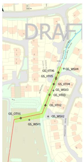
The existing culvert is 525mm in diameter. The proposed upsizing will result in this being replaced by a 1050-1200mm diameter.
