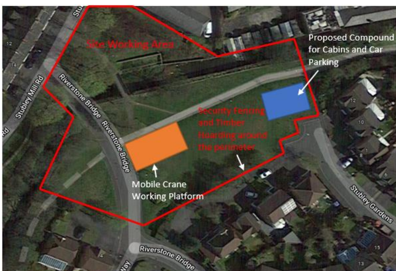
Left: Image showing proposed location of site compound in the Riverstone Bridge green area.
