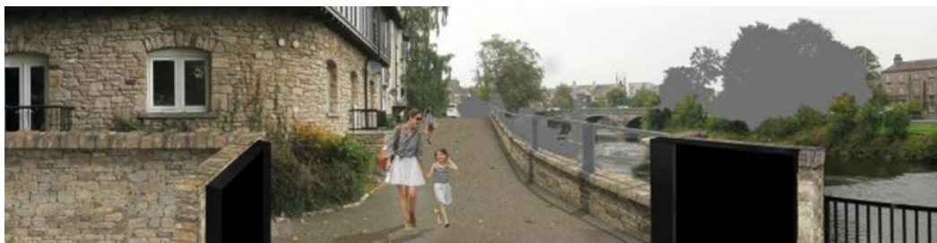
Proposed finish of the glass topped flood wall along Waterside
