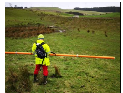
Electromagnetic conductivity survey in progress
