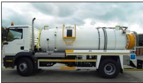
Water jetting tanker
