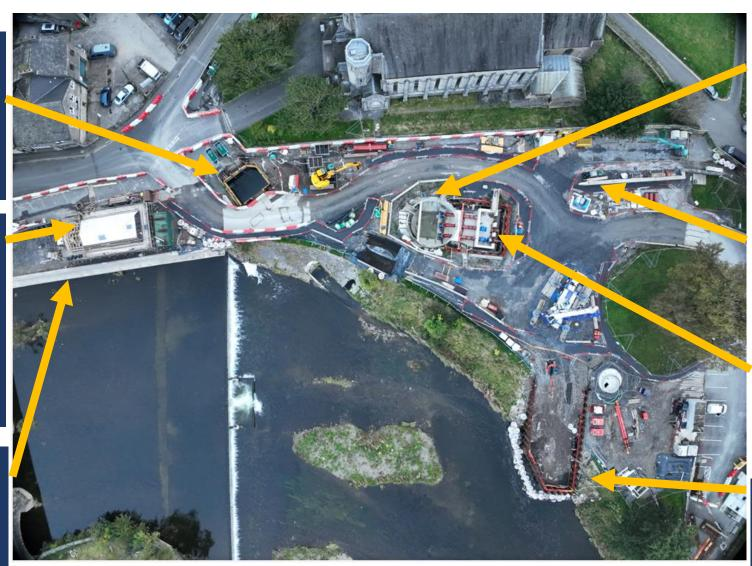
Wet Well – Construction of the underground shaft which will house 3 pumps. In storm conditions these pumps will activate and pump flood water from Stock Beck into the Kent.
