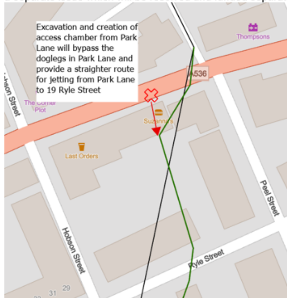
Figure 3 (left): Phase 2 where the excavation from Park Lane (red) is required to connect into the actual culvert line (green) straight on, creating a straighter route for jetting up to 19 Ryle Street. This avoids the doglegs (bends) and steps within the culvert. This will make the jetting more efficient but also safer as there will be a clearer line of sight through the section of culvert being jetted.
