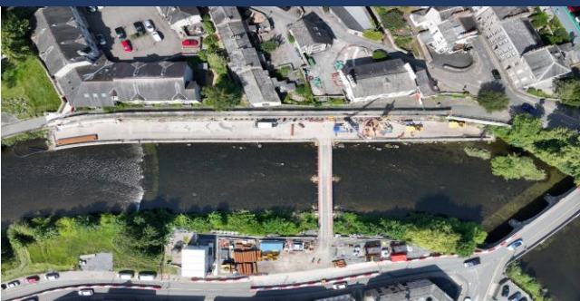
Ariel view of the floating bridge and working platform
