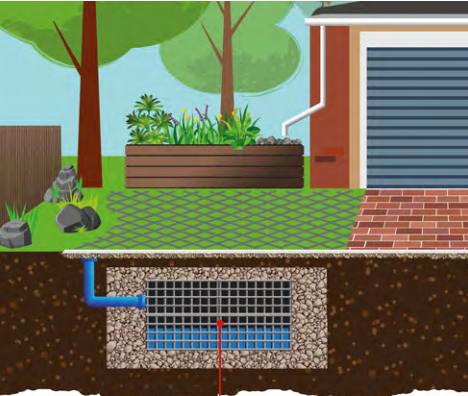
Below ground runoff storage and attenuation crates
