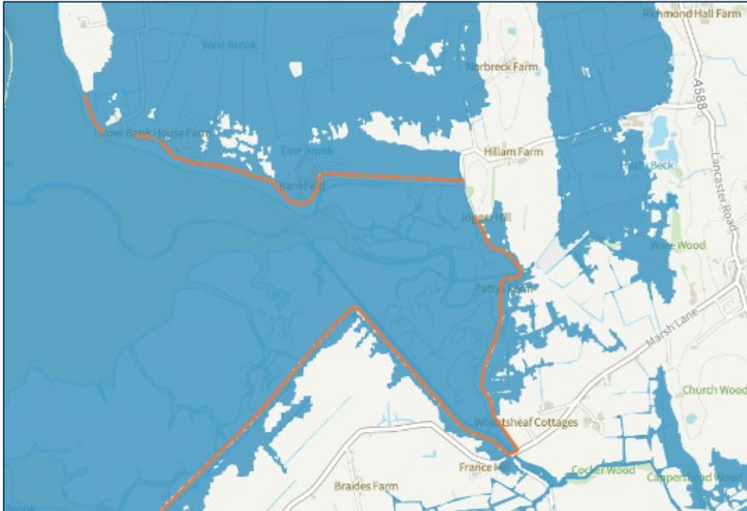
Figure 17 Extent of present-day river and sea flooding with existing defences (1 in 1,000 annual likelihood of occurrence)
