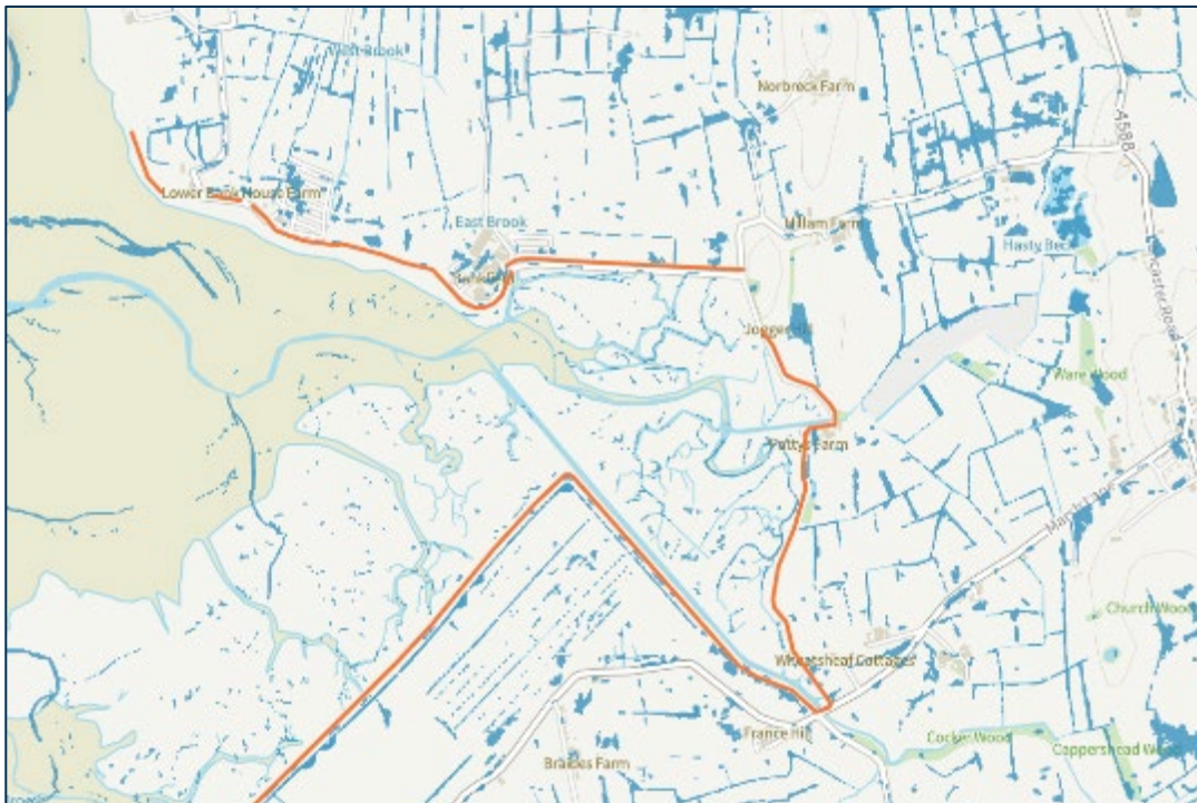
Figure 22 Extent of surface water flooding under a 1 in 1,000 annual likelihood of occurrence
