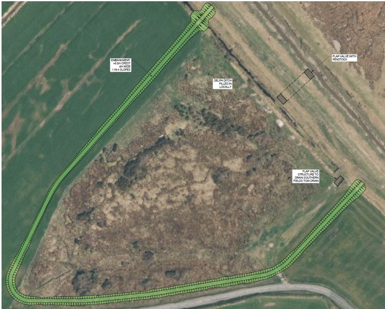
Figure 10 SSSI Option 3a - Regulated tidal exchange
