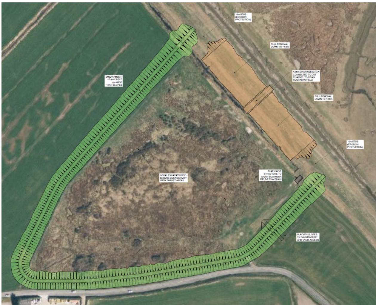
Figure 7 SSSI Option 2a Embankment Removal
