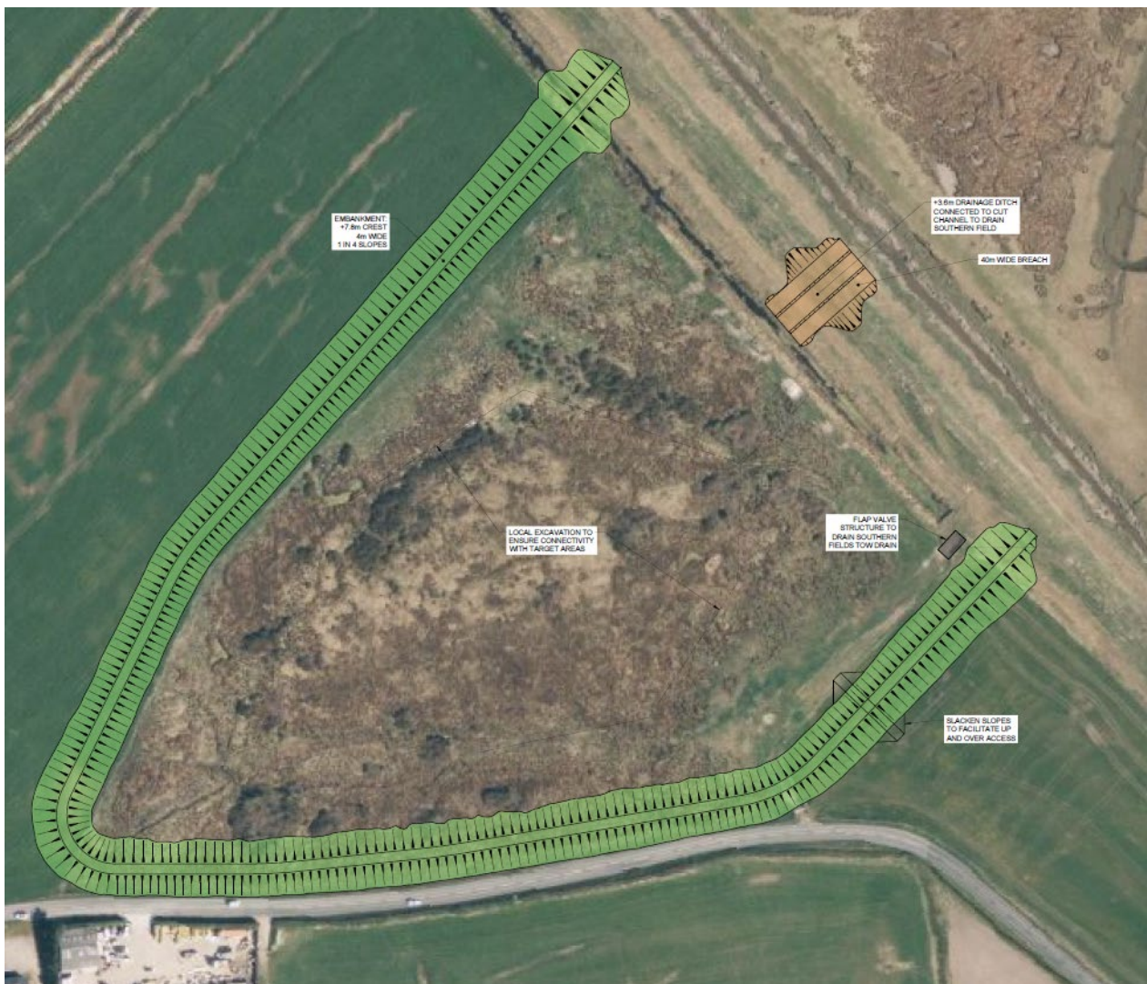
Figure 8 SSSI Option 2b Embankment Breaching
