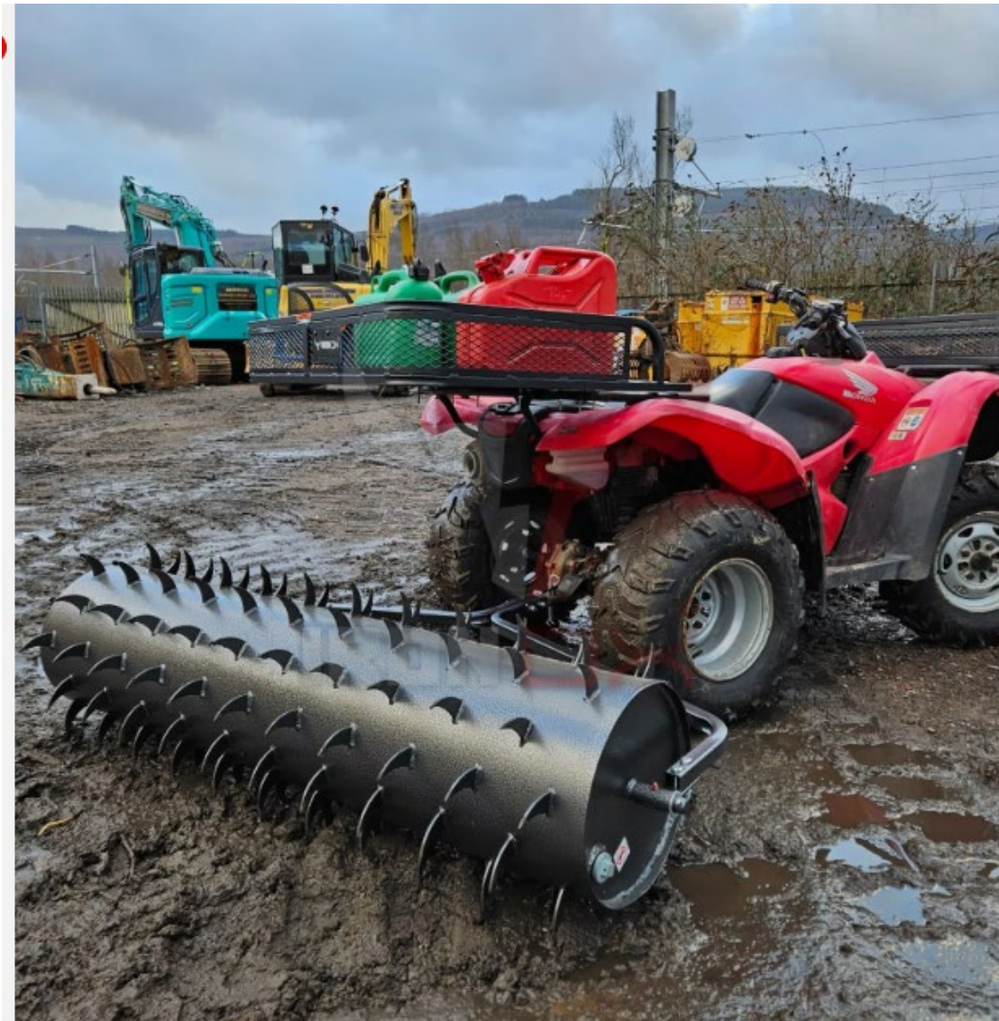
Figure 29. A soil aerator can be used to aerate a field previously subject to heavy grazing pressure and compaction.
