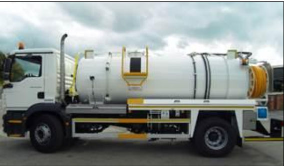
Water jetting tanker
